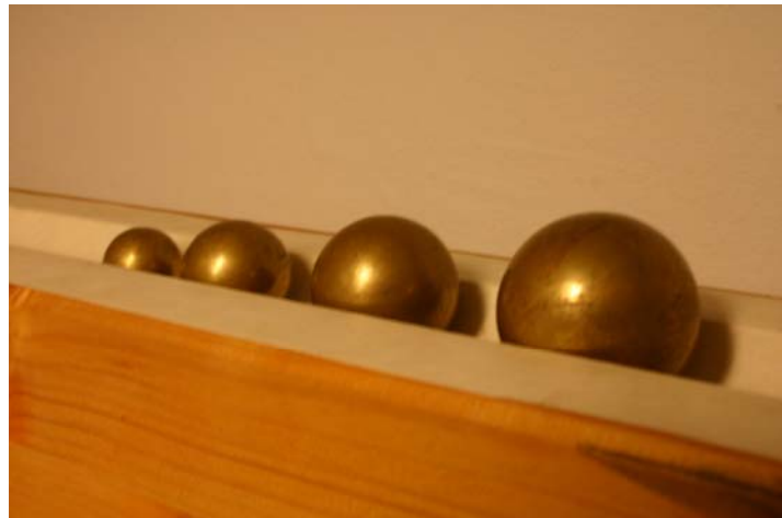
Fig. 3: Brass balls used in the experiments placed in the reconstructed semicircle of the inclined plane
